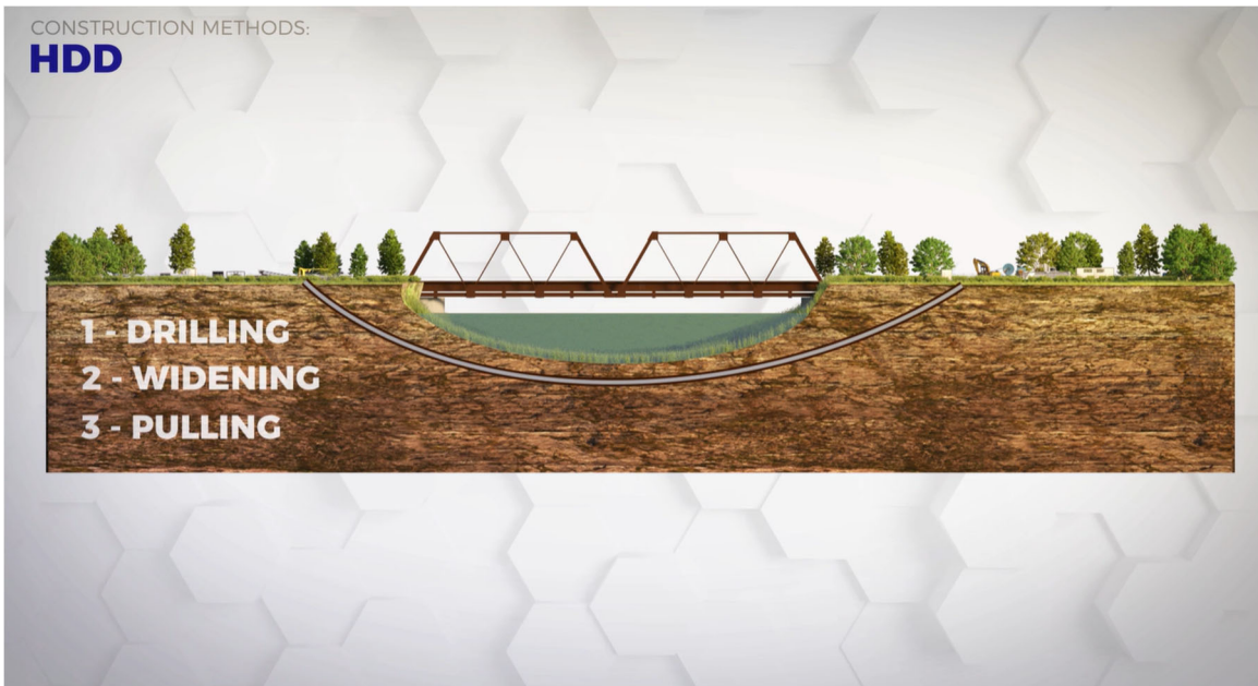
Figure 7-9: Horizontal Directional Drilling Approach
