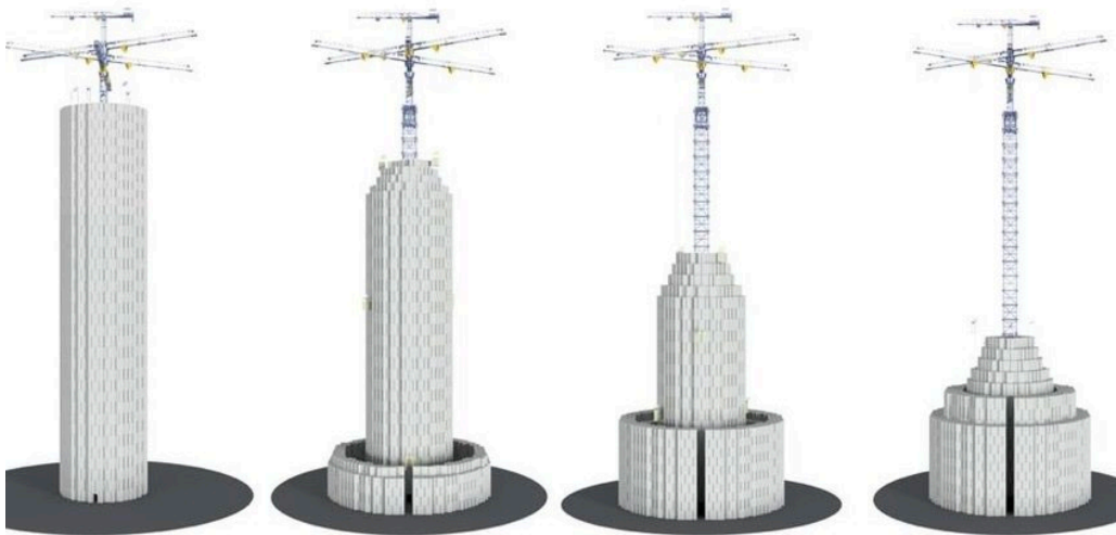
Demonstration of how energy is charged (left) and discharged (right) in Vault (Tower) Energy System [4]
