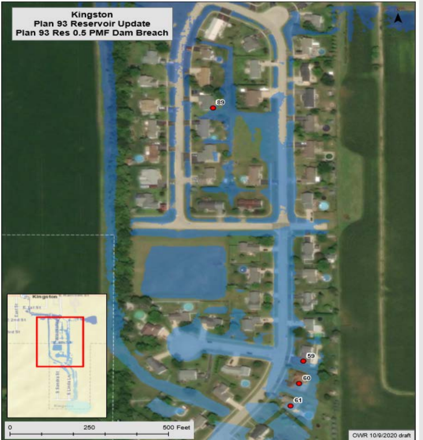
FIGURE 14 - Alternative 3 Reservoir Project 0.5 PMF Dam Breach Damaged Structures Map (Red Dots)
