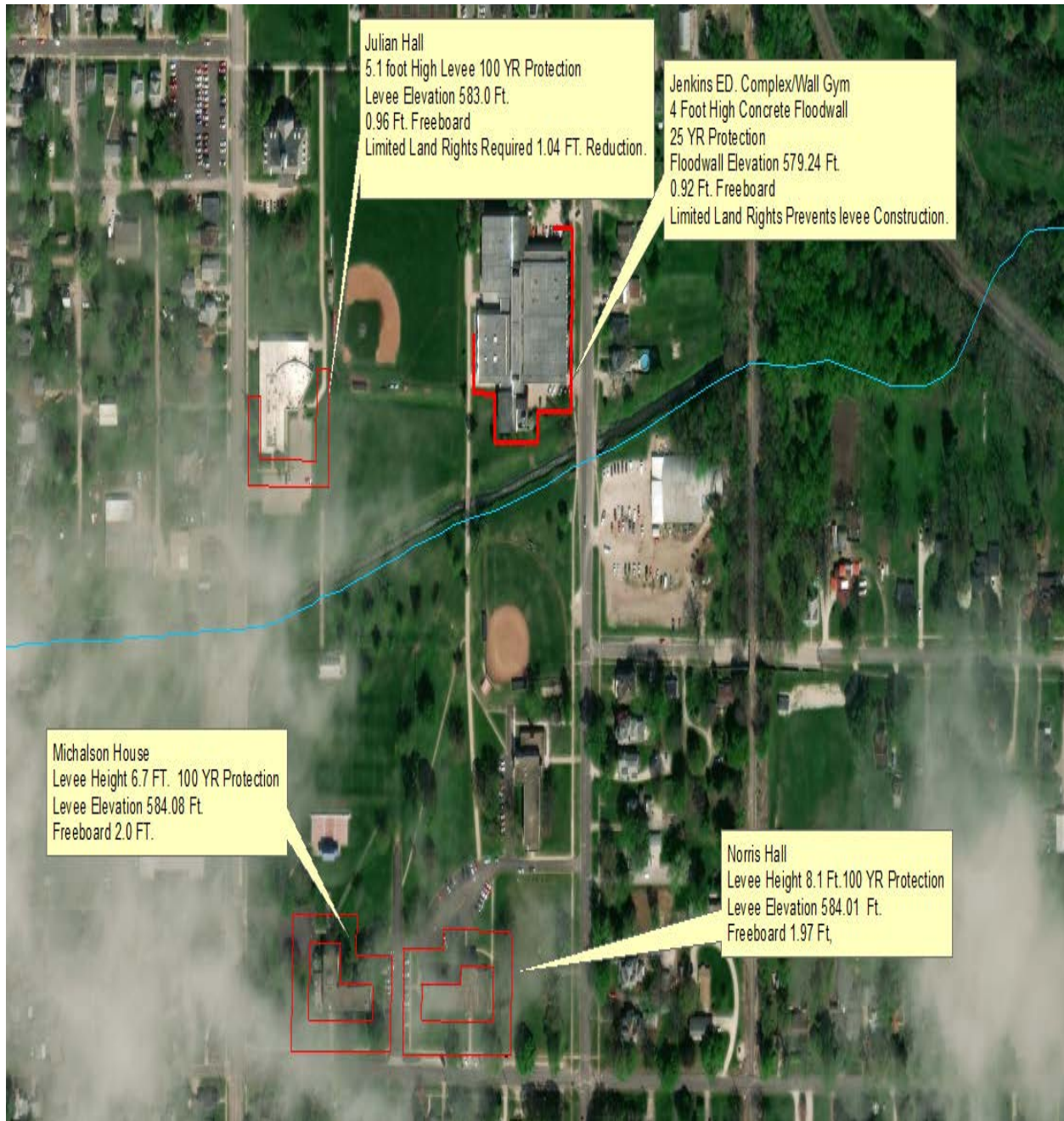
Figure 22 - Alternative 9 – Plan View of Floodproofed MacMurray Structures
