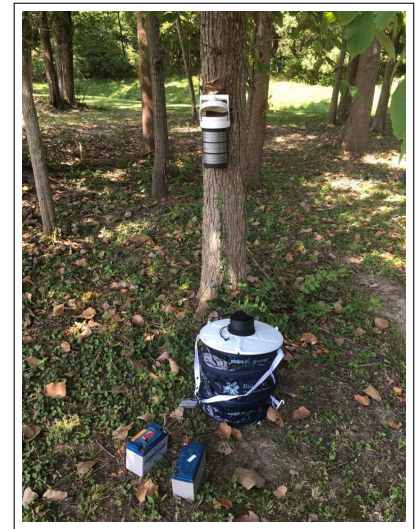
Figure 6: Image of the BG Sentinel trap (on the ground) to collect adult female mosquitoes and an oviposition container (on the tree) used to collect eggs.
